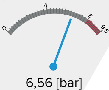
Water pipe pressure - 4-20 mA
