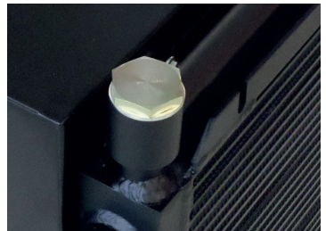
Externer Bypass External Bypass
